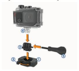
3 Allow the base to bond to the mounting surface for at least 24 hours.
