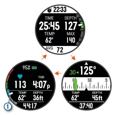
**Dive stopwatch**: Displays the bottom time stopwatch; current, maximum, and average depth; and rate of ascent or decent (*Using the Dive Stopwatch*, page 14).
