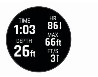
**In-dive screen**: Displays the information about the current dive, including the elapsed time, current and maximum depth, heart rate data, and rate ascent or descent.
