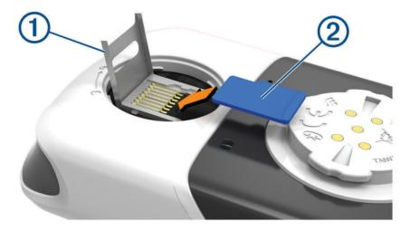
5 Place the memory card 2 into the card holder, with the gold contacts facing down.
