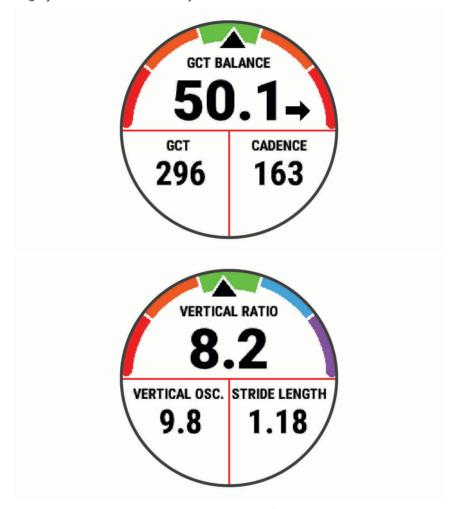
**REMEMBER:** Ground contact time balance is only available if you are using a compatible running dynamics accessory.
