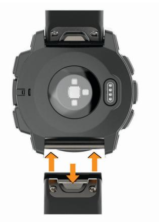
**NOTE:** Make sure the band is secure. The latch should close over the watch pin.
