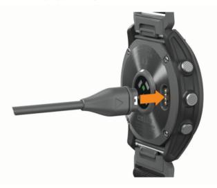
Plug the other end of the cable into a USB charging port. The watch displays the current battery charge level.
