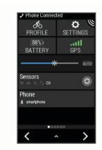
The settings widget appears. A flashing icon means the device is searching. You can select any icon to change the settings.
