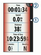
The vehicle position LED ① moves up the column as a vehicle gets closer to your bike. The threat level LED ② changes color based on the potential level of threat. Green indicates no vehicle is detected. Amber indicates a vehicle is approaching. Red indicates a vehicle is advancing at a high rate of speed.
